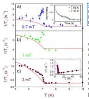
Spin lattice relaxation rate 1/T<sub>1</sub> versus temperature from single exponential fits to relaxation data in the Pb film (260 nm) with implantation energy 5 keV. a)  $B_{ext} = 0.7 \text{ mT, b}$   $B_{ext} = 1\$ \text{ mT, c}$   $B_{ext} = 3 \text{ mT.}$
