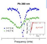
Resonance curves of 8Li ions implanted at 5 keV in Pb with a magnetic field of 1 mT applied parallel to the surface of the film.
