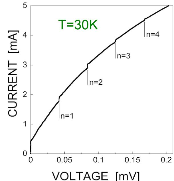
Observation of Josephson current over non-superconducting barrier in pseudogap with  $d \approx 20 \text{ nm}$
