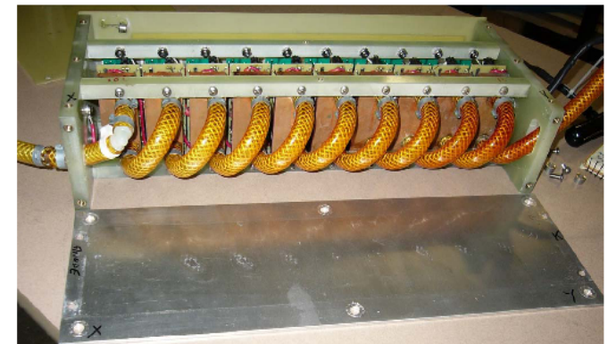
V- On / OFF Switch Hose & Arcing circa 11/2010 after ~1000 hours operation
