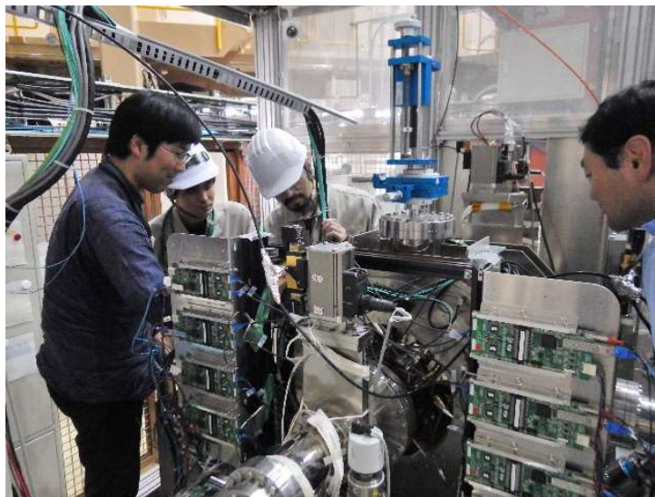
Mr Iwashita, Drs Adachi and Ohishi are preparing the foil sample for the \mu SR measurement.
