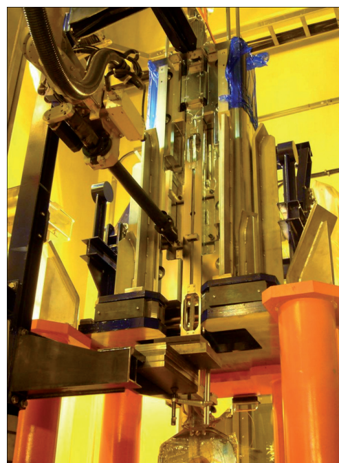
The J-PARC MUSE muon target assembly.
