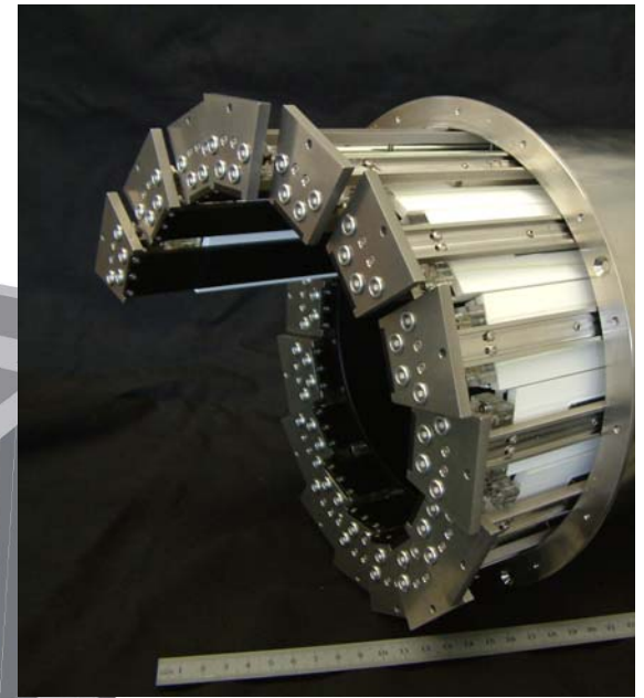
LEM: new positron spectrometer with APD readout
