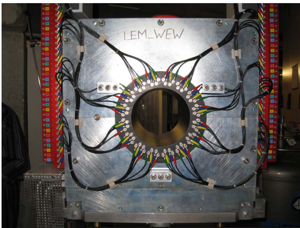
LEM: new positron spectrometer with APD readout
