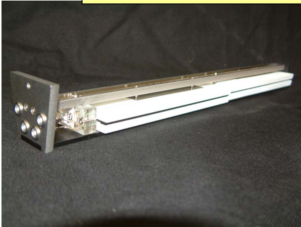
LEM: new positron spectrometer with APD readout
